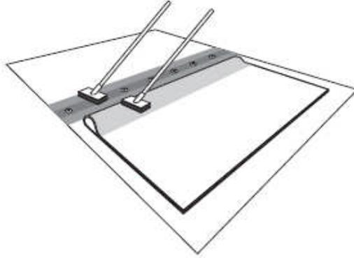
**D. Remove the paper backing:** Allow the Single-Ply QuickPrime Primer to flash off completely. Use the touch-push test to test for dryness. Remove both release papers from the QuickSeam R.M.A. strip and roll the field membrane onto the strip. Use a Stiff Push Broom to ensure an initial bond between the RMA Strip and the field membrane.
