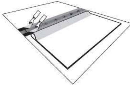
**E. Roll the QuickSeam R.M.A. Strip:** Using a stiff broom Roll the strips using Firestone's QuickRoller across its entire length above both tapes.
